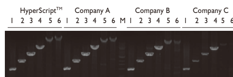
Comparison of HyperScript™ RTase with other companies using primer set of various size. RT-PCR reactions were performed according to each manufacturer's recommendations. Lane 1 : 489 bp Lane 2 : 1024 bp Lane 3 : 2041 bp Lane 4 : 3543 bp Lane 5 : 6936 bp (7 kb) Lane 6 : 9816 bp (10 kb) Lane M : 1 kb ladder
